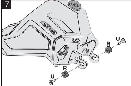
**7** Insert the rubbers (R) (after dismantling them from the original tank) and the bushings (U) before connecting the utilities.
