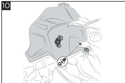
**10** Secure using the original screws (Q) on both sides.
