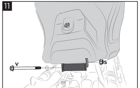
**11** Insert the screw (V) into the appropriate seat screw with the nut (S).
