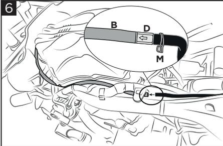
**6** Pull the hose (B) through as shown in figure and connect it to the carbon canister gas' original hose using the valve (D) and the clips (M) .
