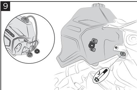
**9** Place the tank on the motorcycle and fix it using the screws (J) on both sides. **ATTENTION:** pass the fuel pipe internally as shown in the figure.
